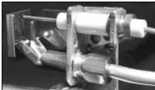
Figure 7 - Ignitor Assembly
